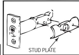
**IMPORTANT:** Do not hammer on latch if bolt is extended. For round face deadbolt installation, no chiseling is required. Simply press deadbolt flush to door edge. Be sure bolt is vertically aligned with door edge (see arrows).
