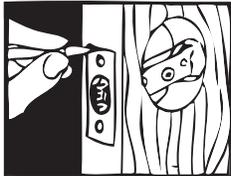
Insert deadbolt into hole and mark outline as shown with pencil. Remove latch.
