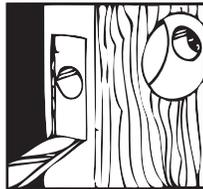
With deadbolt in upright position, attach stud plate and install. Insert two "A" screws and tighten.
